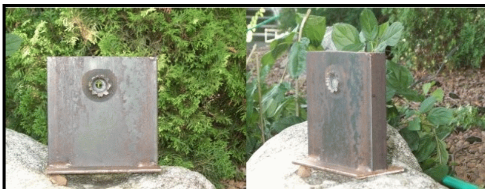
This image from the Internet web site of manufacturer Watson's Weapons shows effect of .50BMG armor-piercing round on one inch steel plate.
