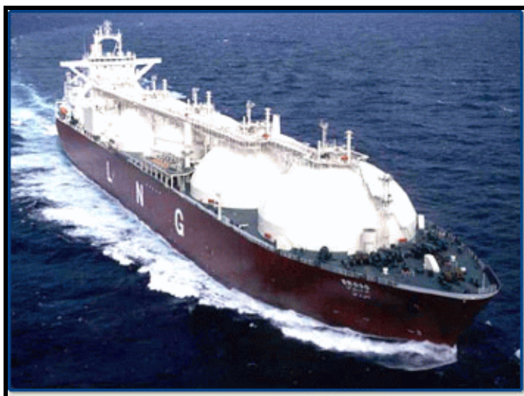
A 50 caliber anti-armor sniper rifle could penetrate the shells of this Moss Rosenberg LNG tanker, according to the Clarke report, but “in all probability” onboard fire fighting equipment could keep ahead of the fires.
